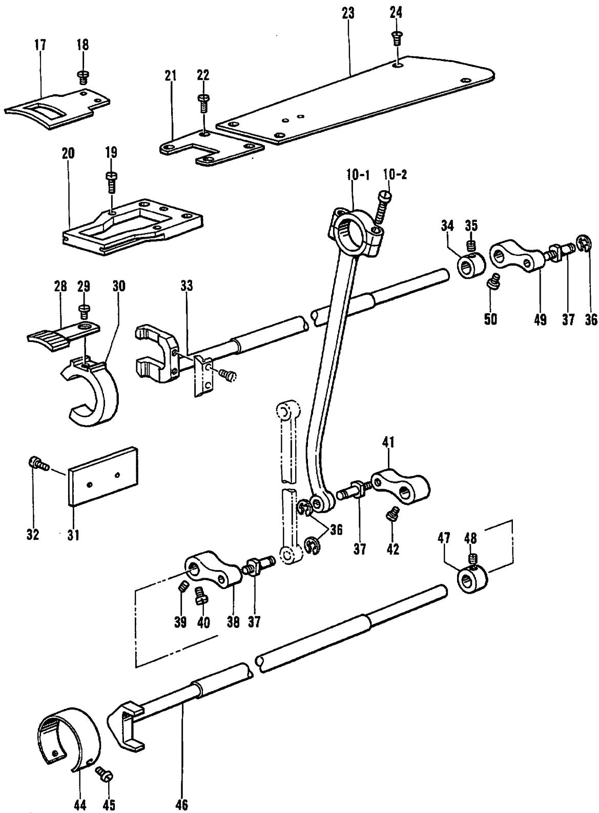
H2. 送り関係 /Feed mechanism/Transportvorrichtung/
