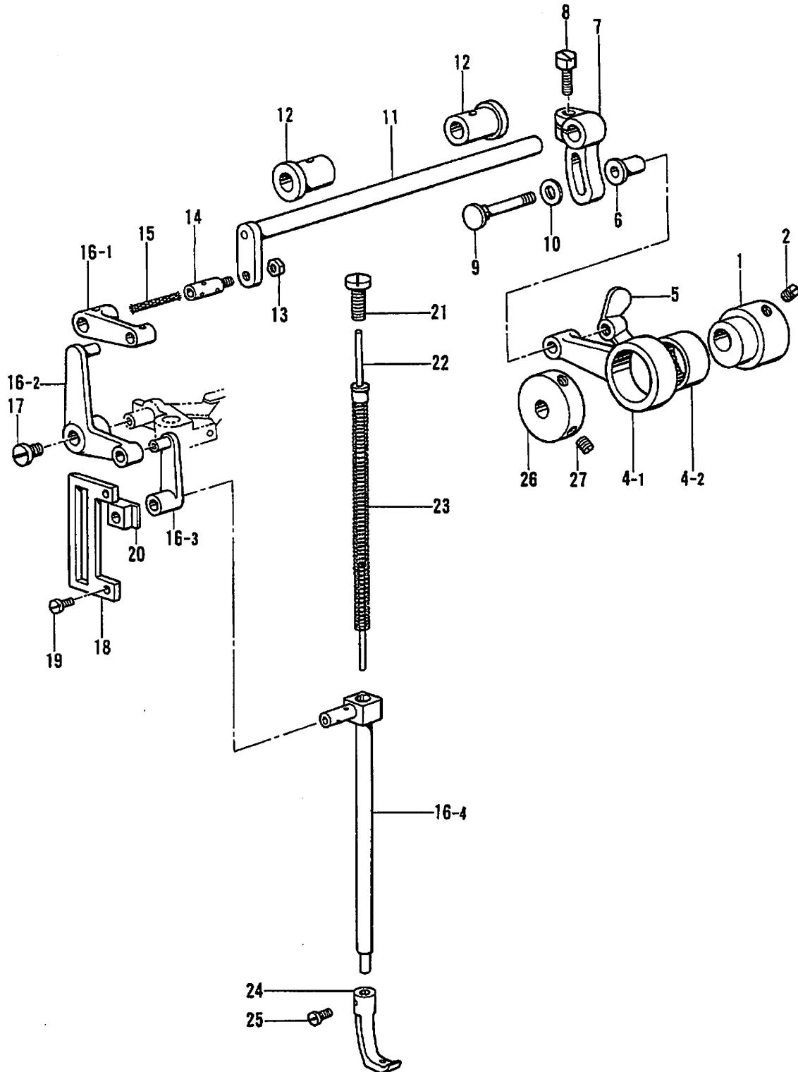
F. 上送り関係 /Upper shaft mechanism/Obertransportvorrichtung/
