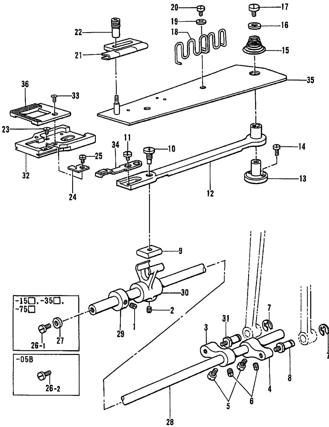
H1. 送り関係 /Feed mechanism/Transportvorrichtung/
