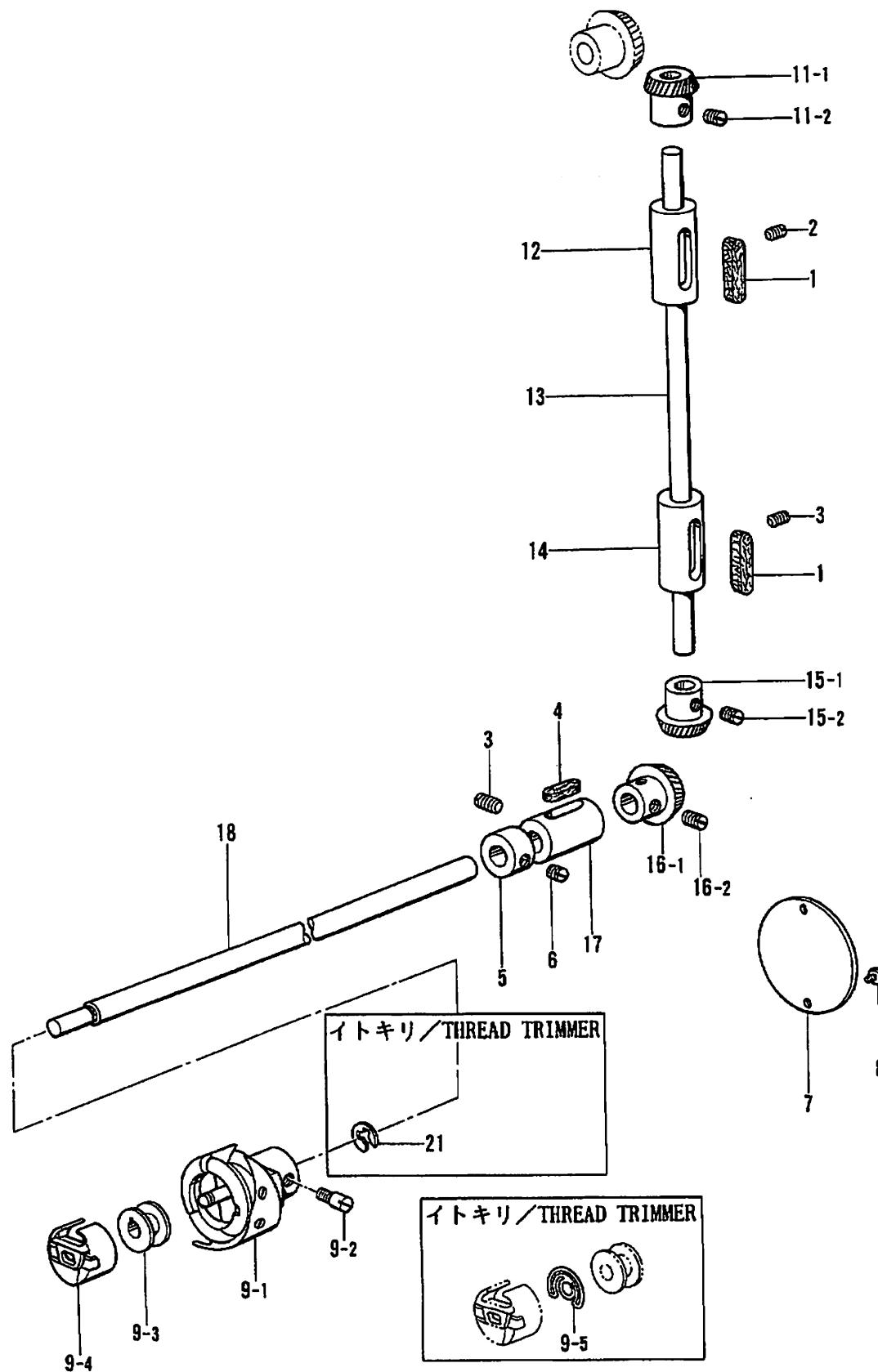
G. 下軸関係 /Lower shaft mechanism/Untere welle/
